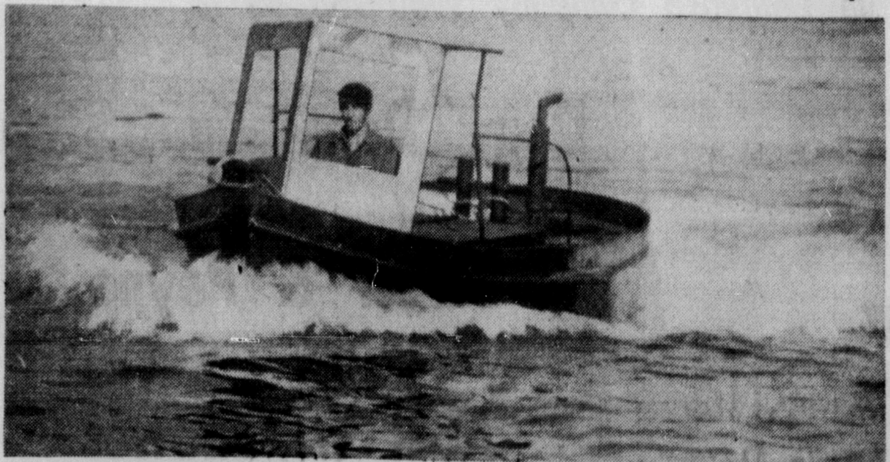
One of five boom boats used by Columbia Cellulose Company in their logging operations. It is 14 feet long and is of all-steel construction. These boats were designed and equipped by US. They carry 110 H.P. Scripps engines.
